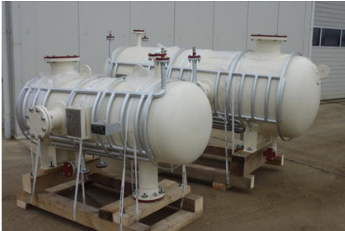
Pulsationdampers for Sour gas application with heating coils
